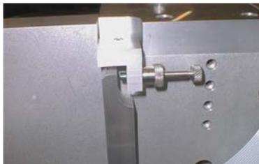
**FEATURES** include programmable speed, default error codes, pneumatic braking of Z and Y-axes during testing and mechanical down stop to keep hook from damaging delicate surfaces. Direct output to a computer via RS-232 interface with capture software. A-1 Feature converts the machine to a peel tester with wire engagement tweezers.
