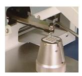
Series 7000C Pull Testers provide an exceptionally convenient means to place a hook under the arch of a bonded wire and then lower the wire under microprocessor control to measure tensile strength, either destructively or non-destructively. Embodied in this series is West-Bond's new three-axis mechanical-advantage manipulator, which is independently guided along each axis, and so is able to transmit motion and force from control to tool undisturbed by loading forces from any other direction.
