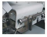
**FEATURES** include programmable dual force (high or low), pure vertical Z, pneumatic braking of all axes during bonding, and radiant tool heat. Available with or without the base and work platform for tabletop or conveyor system applications.
