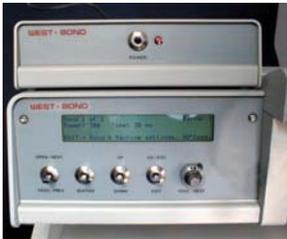
**PROGRAMMING** for thirty different device types may be entered into separate buffers. Each device wire may have up to 21 stitch bonds with individual ultrasonic power, time, force (high or low) and loop elevation control data. Program values, action prompts, and fault diagnostics are exhibited on the easy to read 4 line, 40 character LCD sequentially with machine operation.
